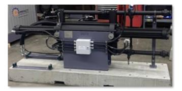
At the conclusion of our 3-year test program, our newly designed coating, **CCI-SS (Seal Saver)**, has produced impressive results. The increased life expectancy of rods coated with CCI-SS is yet to be determined, as none have shown significant wear, even in harsh environments with production chemistry, contaminants, and higher levels of solids production. To date,
